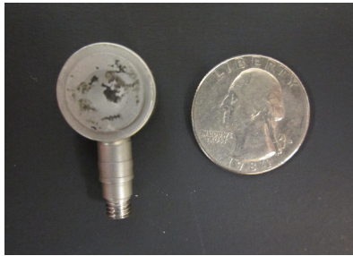
Figure H.1 Force transducer employed in impact experiments.
