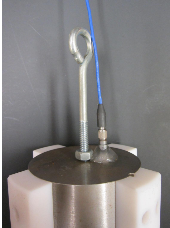
Figure H.4 Impactor with accelerometer attached.
