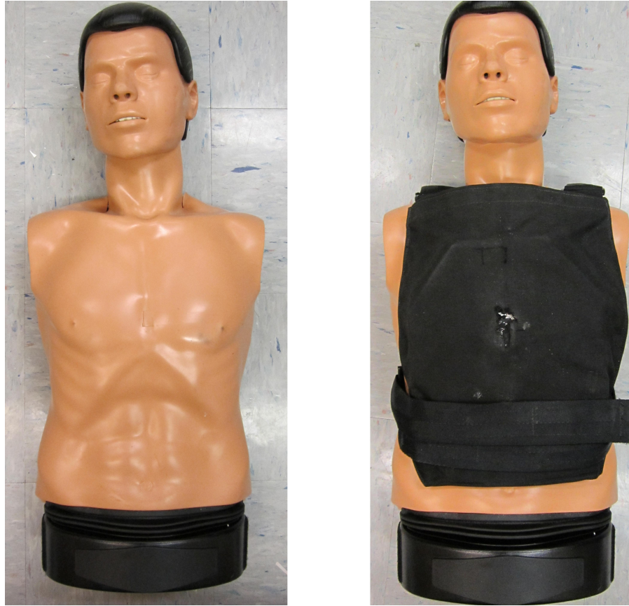
Figure 3.3 CPR manikin employed during impact testing. Left: manikin without vest. Right: manikin with carrying vest and armor plate.
