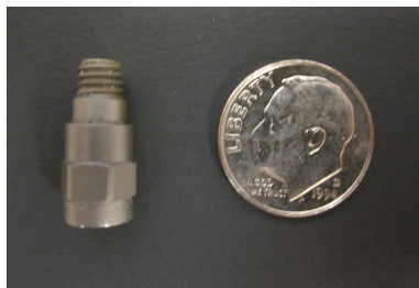
Figure H.2 Accelerometer employed in impact experiments.
